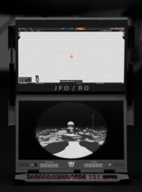
The Joint Fire Observer / Remote Observer station is intended for an operator supporting the mission conducted by JTAC on the basis of applicable support procedures in accordance with the scenario established by the Instructor.
